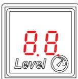
**All segments are on:** no connection or software level sensor function is disabled
