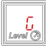
**Blinking "G" symbol:** low gas level in tank or waiting to start operating mode.
