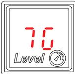
**"Shifty snake", stays on "G":** Etalon measurement process of a gas tank capacity is in progress.
