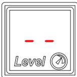
**Stays on two dashes:** engine runs on LPG, waiting to start for etalon measurement.
